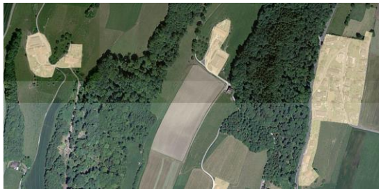
Figure 4-6 The perimeters are entered on the basis of the aerial image depicting the developed area. The z values are automatically transferred during digitisation from the digital terrain model to the base points of the development contours.
